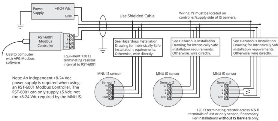
Modbus System Wiring with RST-6001
