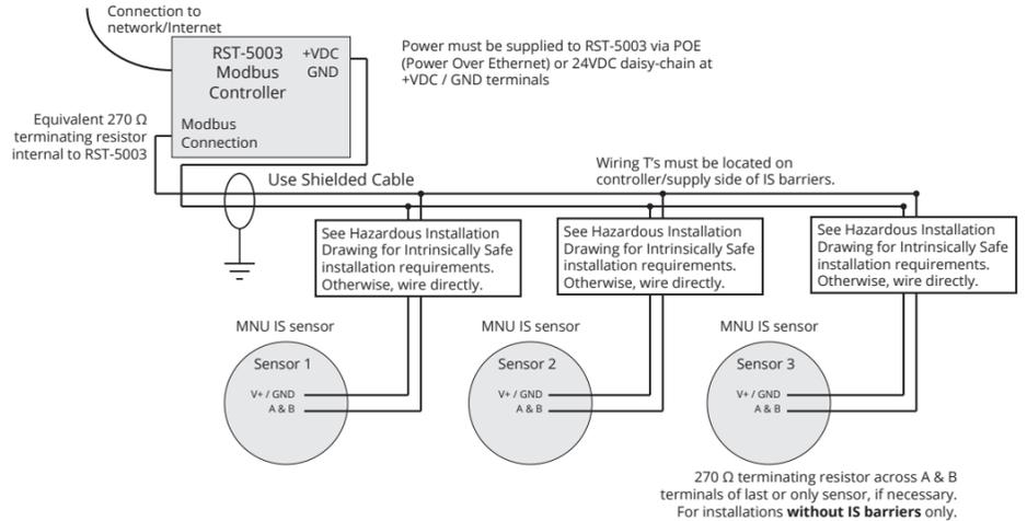
Modbus System Wiring with RST-5003 and Power Over Ethernet (POE) or VDC
