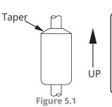
♠ IMPORTANT: Floats must be oriented properly on the stem, or sensor readings will be inaccurate and unreliable. Untapered floats will have a sticker or etching indicating the top of the float. Remove sticker prior to use.
