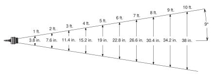
Typical beam spread of a sensor operating at maximum sensitivity
