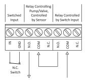
Trip 1 (NO) is controlled by the sensor (see Relay Trip Types and Relay Logic Diagrams on pages 32-33), closing for ON conditions. Since Trip 2 is also NO, both trips must be active (ON) for the Pump/Valve circuit to be complete.
