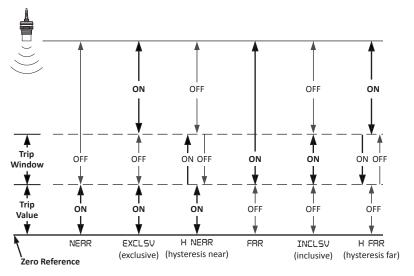
Relay Logic for all Volumetric Modes
