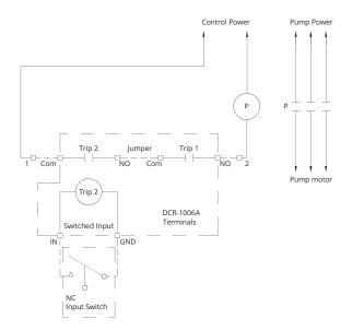
DCR Switched Input as Start Prevention Control Wiring
