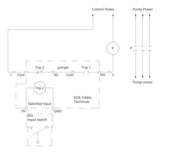
DCR Switched Input as E-Stop Control Wiring
