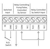
Trip 1 (NO) is controlled by the sensor (see Relay Trip Types and Relay Logic Diagrams on pages 32-33), closing for ON conditions. If the NO input switch closes, Trip 2 will open, breaking the circuit through Trip 1.
