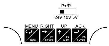
Figure 6. Transmitter Supply Voltage Selection
