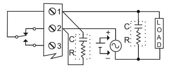
Figure 13. AC and DC Loads Protection
