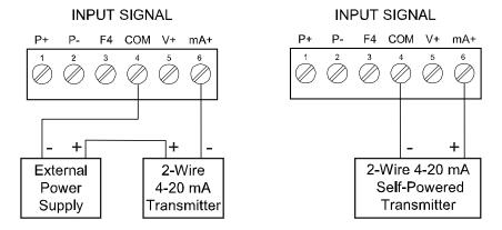
Figure 10. Transmitter Powered by Ext. Supply or Self-Powered
