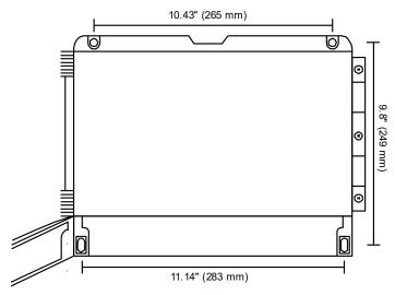
**Figure 1. Meter Mounting Holes**
