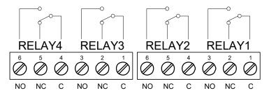
Figure 12. Relay Connections
