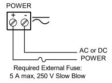
**Figure 8. Power Connections**
