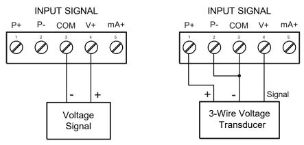
Figure 11. Voltage Input Connections
