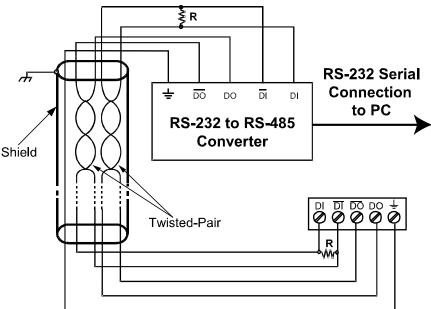
Figure 15. RS-422 or RS-485 Wiring
