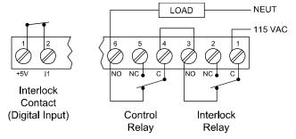
Figure 22. Interlock Connections
