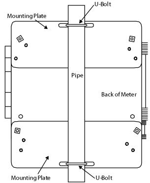
Figure 4. Vertical Pipe Mount Assembly
