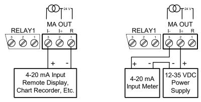
Figure 21. 4-20 mA Output Connections
