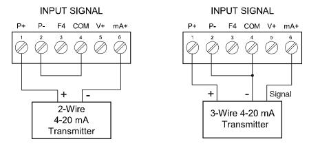
Figure 9. Transmitters Powered by Internal Supply
