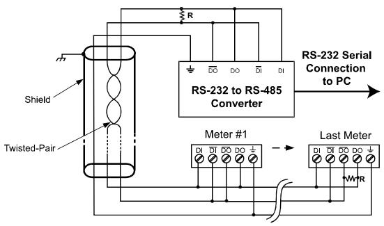
Figure 16. RS-485 Two-Wire Multi-Drop Wiring
