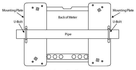
Figure 5. Horizontal Pipe Mount Assembly
