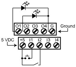
Figure 19. Digital Input and Output Connections
