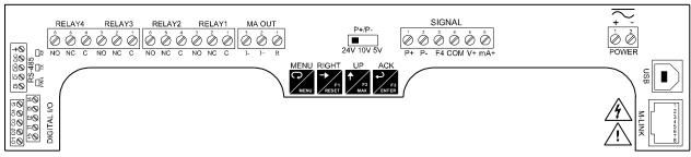
Figure 7. Connector Labeling for Fully Loaded Meter
