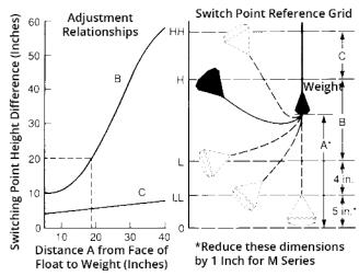
that the pump "off" position (level L) is 15 inches from the bottom of the tank. This means that the float must be hung so that the zero reference height (free-hanging face of the float) is 6 inches from the bottom of the tank. The high and low alarm points HH and LL will then be, respectively, close to 41 and 11 inches from the bottom of the tank.
