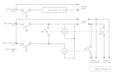
Note: Usually an alternator control is added to the lead and lag pump control circuits. This control automatically alternates the order in which the two pumps come on. In this way the wear on the pumps is evened out. If this is not done, in the course of time, the user will have one (lead) pump that is well worn and one (lag) pump that is barely used. If the pumps use three phase power, the single pole switch contacts, R1B and R2B, would need to be heavy duty three pole switch contacts.
