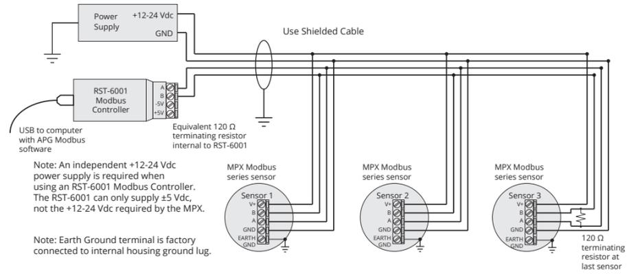
**IMPORTANT:** For EMI protection, either connect the grounding screw (see section 4) to an earth ground, or ensure that tank mounting of the MPX is grounded.
