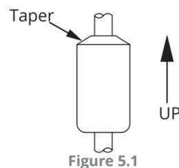
**IMPORTANT:** Floats must be oriented properly on the stem, or sensor readings will be inaccurate and unreliable. Untapered floats will have a sticker or "N" indicating the top of the float. Remove sticker prior to use.
