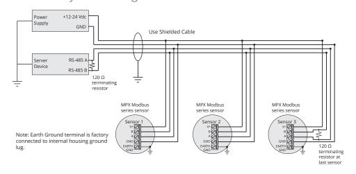
● IMPORTANT: For EMI protection on an MPX-E4 or -R4, either connect the grounding screw (see section 4) to an earth ground, or ensure that tank mounting of the MPX is grounded.
