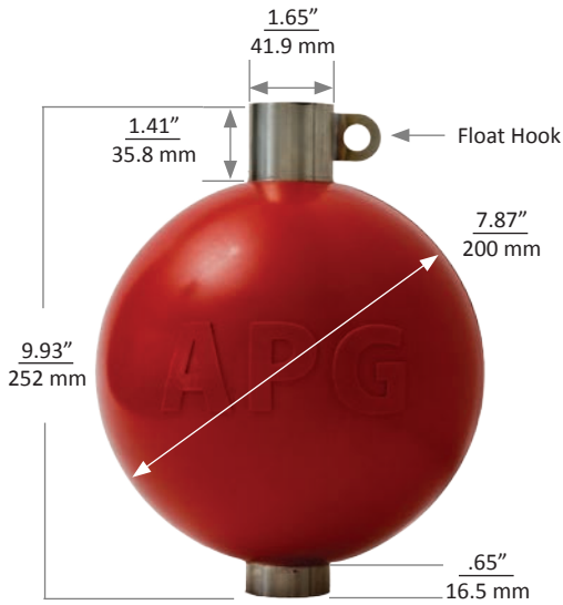
Float F - Polyurethane with 316L Stem (0.44 SG)
