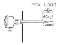
• The maximum length for the threaded boss/mounting nozzle is 70 mm. If exceeds 70 mm, the sensor will detect the dead stock despite there aren't any measuring materials in case of horizontal mounting.
