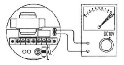
After adjustment, set the switch to H or L and make sure 8~10 VDC can be read.
