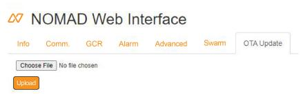
This tab is used to update Nomad Firmware Over the Air, via Wi-Fi. This procedure should not be attempted without APG consent, and only with a firmware specifically made for it.
