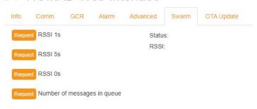
Function 1: Request the RSSI for Swarm. The RSSI is the signal to noise ratio. After installation and during configuration, please hit "Request" in front of "RSSI 1s" to display the signal to noise ratio. The value will be displayed at the bottom of the screen.
