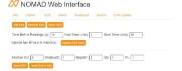
**Time Before Readings (s)** is used to tell Nomad how many second(s) a reading will be accessible on the slowest sensor connected to it. For example, if the slowest sensor takes 10s to transmit a correct reading after powered up, please enter at least 10 in this box.
