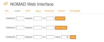
Before you begin connecting your sensors to Nomad, you must ensure it is communicating at the same rate as Nomad. Standard Nomad communication is 9600 Baud, 8 bits, 1 Stop bit, No parity. Information for your specific sensor can be found in your sensors' user manual.
