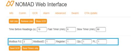
The line inside the blue box controls what Nomad does on a regular basis. Each command is on a separate line. Additional lines can be added by clicking on the **Add Line** button.
